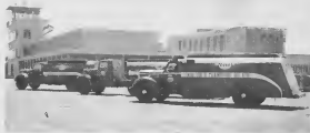
On display at Dakota, with the operations tower as a background, are the three big trucks which help to service the planes. In the center is Lago's bulk hauler which brings high-octane fuel from the refinery to the field. Bracketing it are two aviation refueling trucks, which can deliver at the rate of 180 and 100 gallons per minute.
